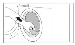
Fill the smaller upper hole and the two large ones with the corresponding plastic plug caps supplied in the bag containing the instruction booklet.
